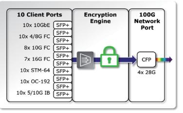
make the difficult choice between running unencrypted at 100G, or link aggregating 10 x 10G encrypted ports. Well, Big Data is no longer in that difficult position, as the ADVA FSP 3000 supports both 10G and 100G in-flight, bulk encryption. Any combination of protocol and data rate can be grouped together and transported with 100% throughput over a channel.
