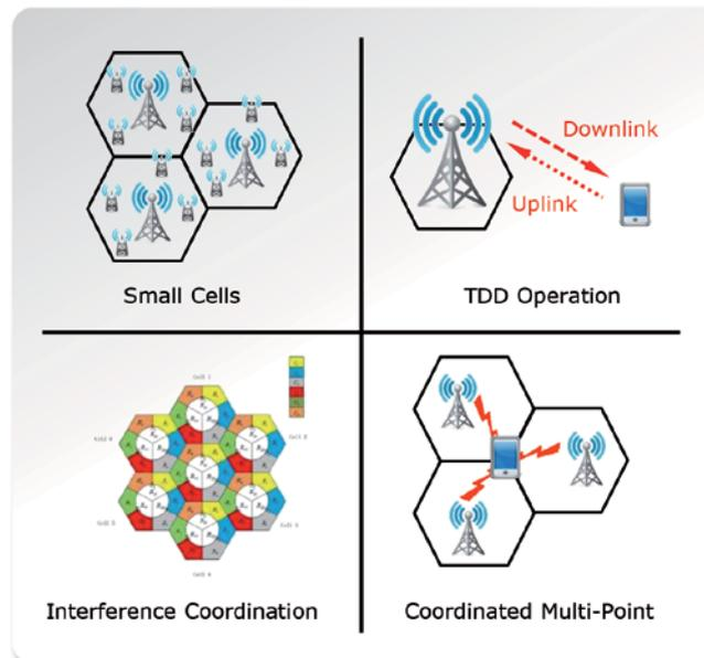
Both TDD operation and eICIC need base stations to be synchronized with respect to the up- and downlink transmission times. If neighboring base stations use different time assignments and share the same spectrum, then interference between cells may occur.
