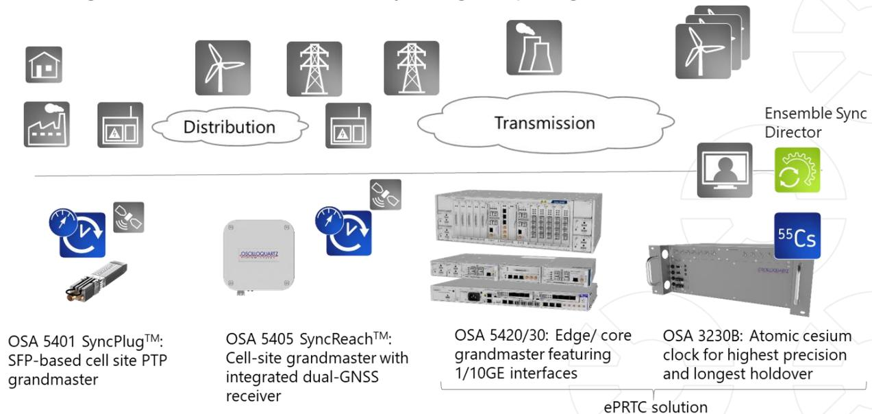
The OSA 5420 is an essential component for timing excellence in energy distribution networks. It supports the widest range of interfaces as well as multiple PTP profiles including power profile, and can be applied as a gateway between telecom and enterprise timing networks. What's more, in the core of the network, our OSA 5430 and OSA 5440 in combination with our cesium atomic clocks provide unique standards-compliant enhanced primary reference time clock (ePRTC) accuracy.
