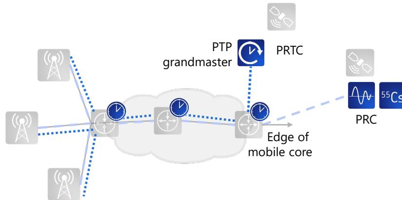
Cell site timing with  $\mu$ s accuracy
