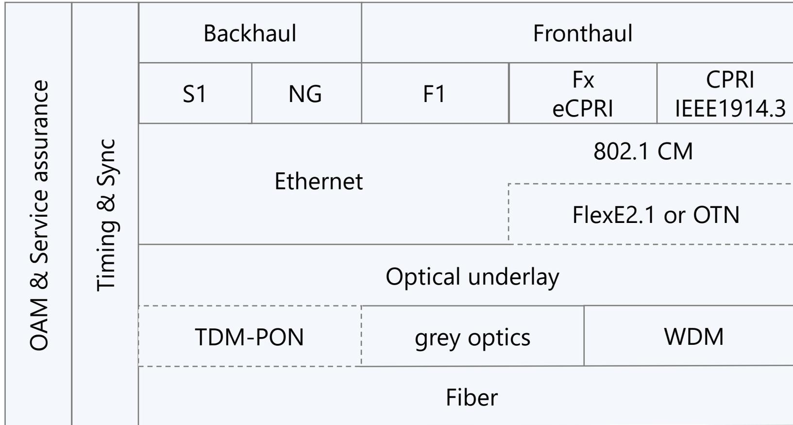
Ethernet is simplest. TDM-PON, FlexE and OTN add additional protocol layers.
