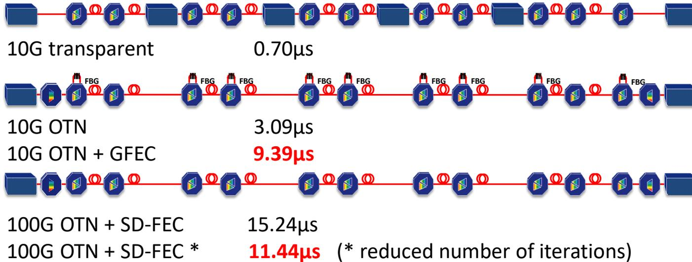
10 span system, 20dB loss per span
