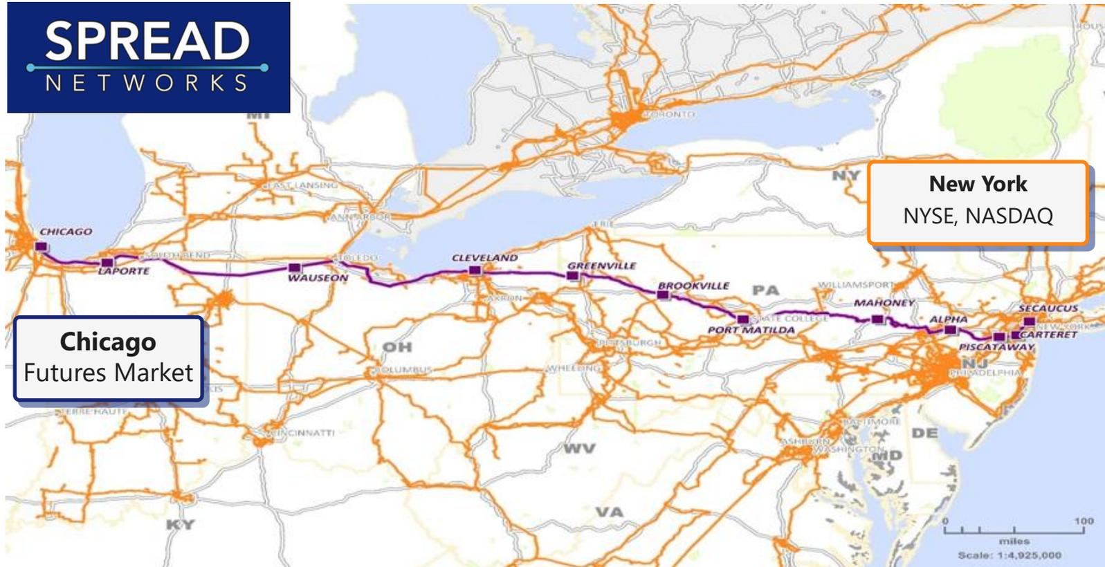
Latency close to fiber propagation delay ( $5\mu\text{s}/\text{km}$ )
